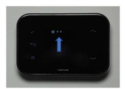
8. On the thermostat, the WiFi Antenna will flash until the devices are successfully paired, at which point the Antenna will remain solid without flashing.
