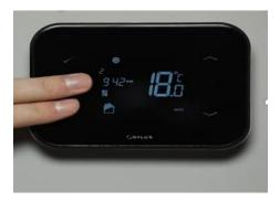
4. On the thermostat press and hold the cog key and return key at the same time.
