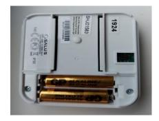
1. Remove the battery cover and insert 2 x AAA Alkaline Batteries into the iT300 Sensor.
