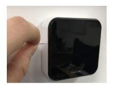
2. Insert a paperclip, pin or similar into the hole on the left hand side of the sensor for 2 seconds until the red light starts flashing.
