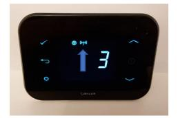
10. Once the Wifi Antenna has stopped flashing your devices are paired even if the 10 minute countdown has not completed. To exit pairing press the return key until the home screen appears.
